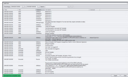
The GxP Module offers all functionalities that are needed for CFR compliance, such as an audit trail of all user activities.
