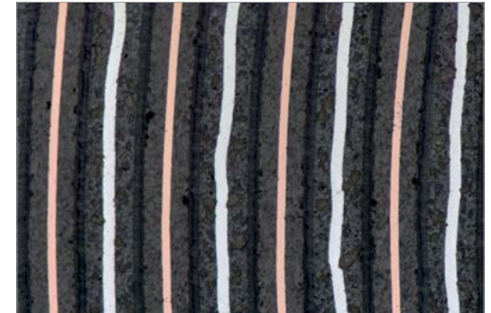
Lithium ionic accumulator, 112x, brightfield
