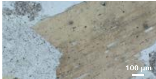
Biotite inside granite, transmitted light, bright field, EC Plan-NEOFLUAR 10x/0.3 Pol
