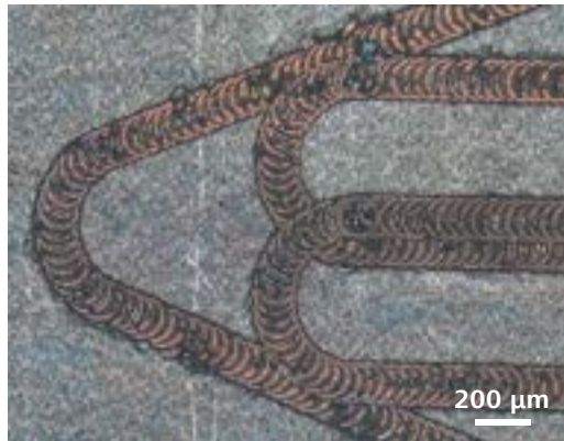
Milling marks for engraving purposes, EC EPIPLAN 5x/0.13
