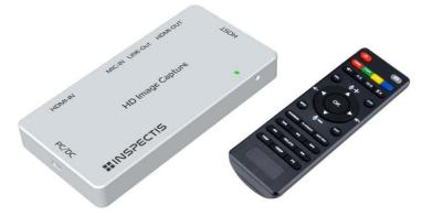
Compatible with HD (720p), Full HD (1080p) and 4K (2160p) output signals of Inspectis Digital Microscopes. Captures live video and still pictures up to 1080P resolution (1920x1080 pixels) via USB flash drive interface without need of host computer.
